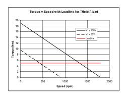
The actual operating point is found at the intersection of the load-line and the motor characteristic for a given terminal voltage. It can be seen that if the terminal voltage is increased, the motor accelerates until it settles out at a new higher speed and depending on the type of load-line – possibly also a new higher load torque.
